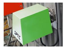
With the fully integrated fail safe shutter the P-5FA is optimally protected for reliable use even under overpressure conditions.
